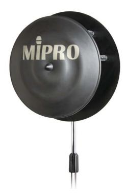
The MIPRO AT-100, Circularly polarized antenna, is a highly directional solution for both transmitting and receiving RF signals across the UHF 470-1,000 MHz bandwidth with up to 8 dBi antenna gain. The AT-100's directional focus in the vertical and horizontal planes effectively reduces the polarization loss of the antenna improving signal strength and signal stability. It's antiinterference performance reduces RF interference and signal drop-outs.
