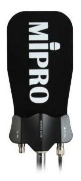
The AT-70Wa is a bi-functional log wideband omni antenna for professional receiving and transmitting. It enhances signal pickup and transmission for MIPRO UHF wireless receivers operating in the 470MHz to 1GHz frequency range and is compatible with US FCC regulations. It has 2 - 4dBi gain which is ideal for any specific installation requiring remote omni antennas.
