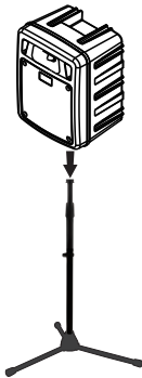
Installed on a tripod
